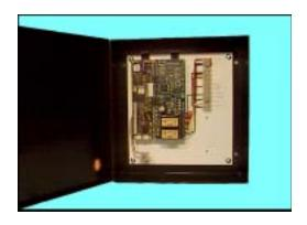
Congratulations you have just purchased the INTELLIKEY Door Control Unit or DCU for short, INTELLIKEY part number 100323. The INTELLIKEY DCU has been designed for controlling a magnetic lock, an electric strike, electrified hardware or almost any other type of electrified device. Not included with the DCU are the needed locking devices or the regulated power supply with battery back up.
